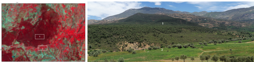
Figure 2. False-colour composite (bands of 5-4-3 NIR, Red and Green) make Cannabis plants appear bright red because they reflect infrared light strongly (upstream of study area – rural commune of Bab Taza)
